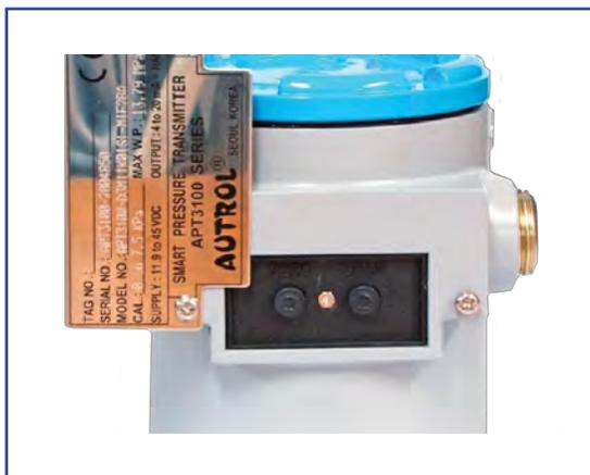
To access the magnetic push buttons loosen one of the screws holding down the nameplate on the top of the transmitter. Turn the nameplate out of the way; underneath are two push buttons labeled Zero and Span. These magnetic push buttons are fully functioning (see menu tree in following pages).
