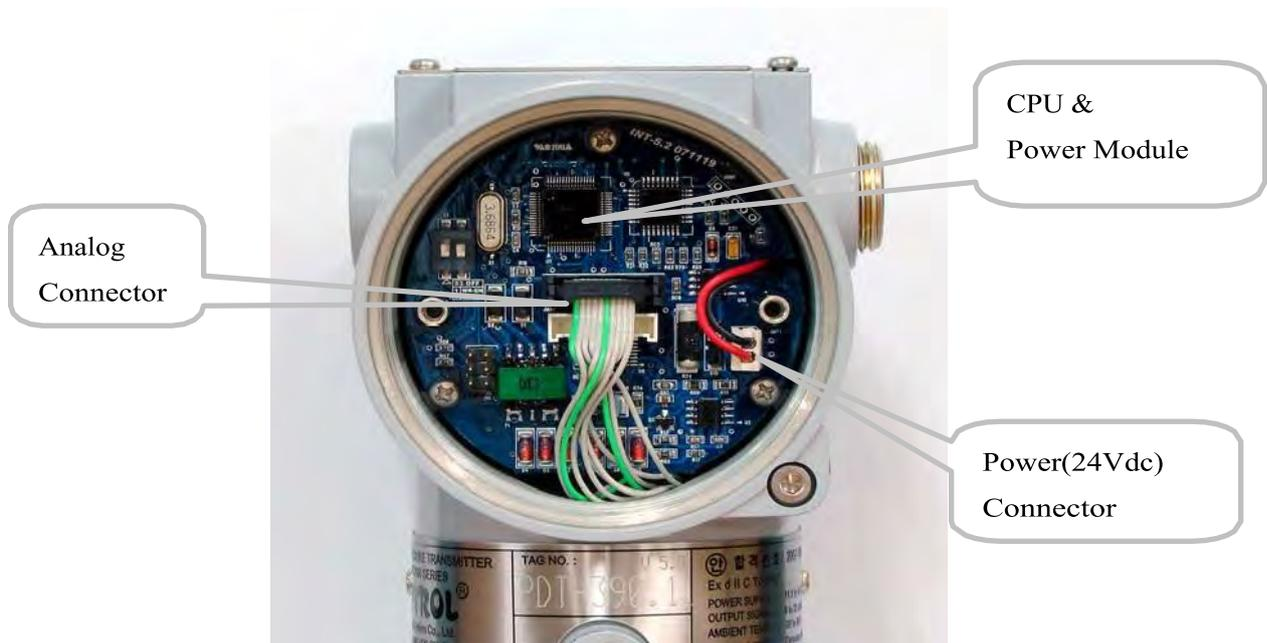
Figure 6.3 Structure of Electronics Module inner Transmitter
