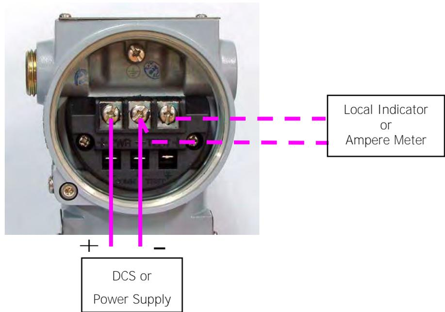
Figure 4-3 Picture of Terminal Board of Transmitter
