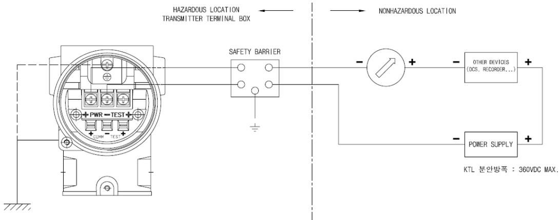
[Figure 4-3 Connection between Transmitter and Power Supply]
