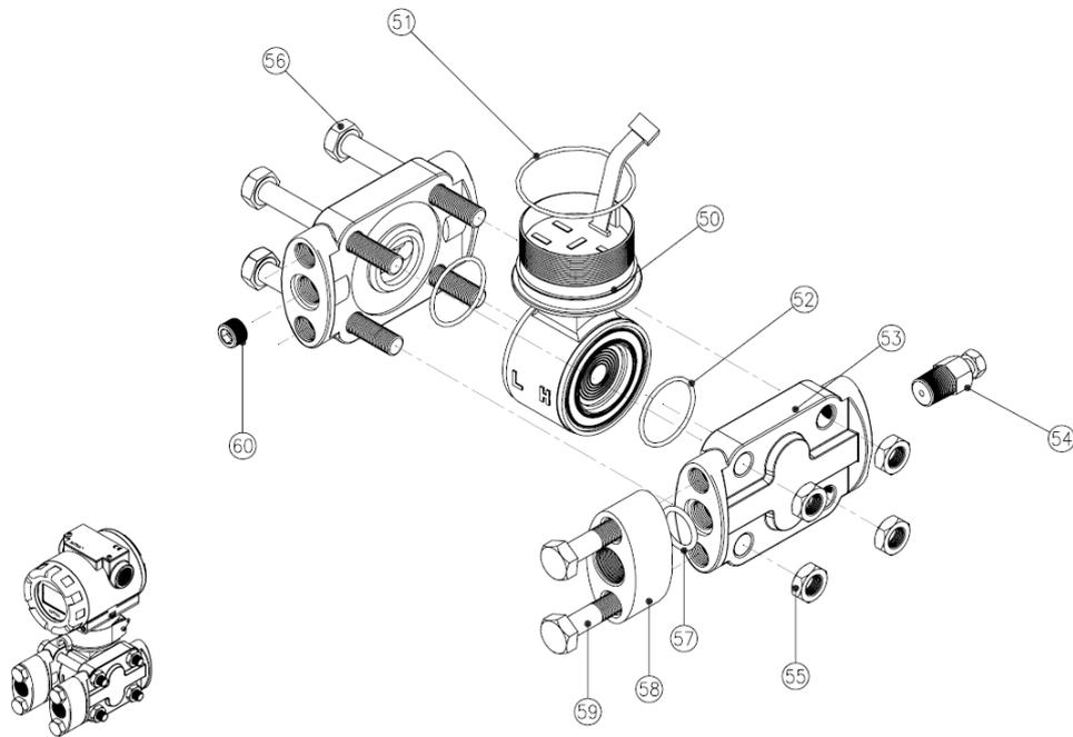
Figure 1-3. Model **APT 3100** Exploded View (Sensor Module-D,G,L)
