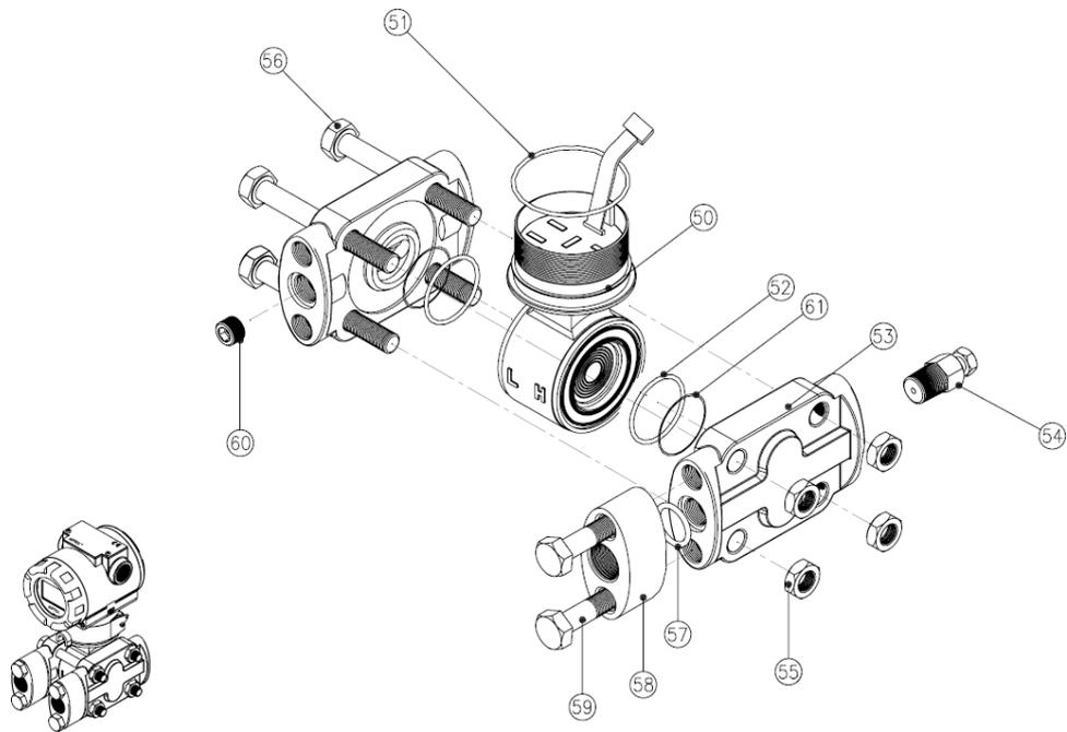
Figure 1-5. Model **APT 3100** Exploded View (Sensor Module-H)
